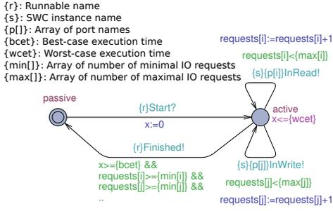
**Figure 3: Schematic description of an UPPAAL TA realizing the behavior of a Runnable implementation ①.**
