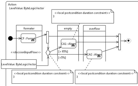
**Figure 6: Flow processor component activity diagram.**
