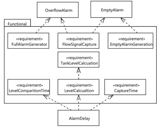
Figure 4: Sugar cane system functional requirements
