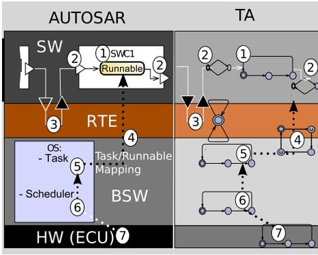
Figure 1: The AUTOSAR layered architecture.
