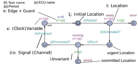
Figure 2: Schematic description of a UPPAAL TA realizing the behavior of an OS task.
