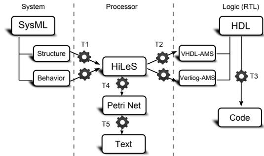
Figure 1: HiLeS Model transformation chain
