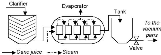
Figure 3: Sugar cane process
