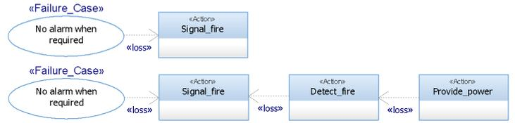
Figure 5: FDS failure case 1 - before and after expansion
