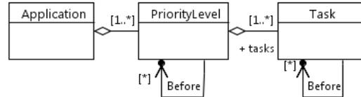
Figure 4. Verification-oriented meta-model
