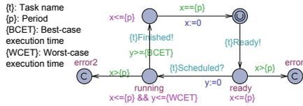
**Figure 11: Schematic description of a UPPAAL TA realizing a task simulating a part of the remaining system.**
