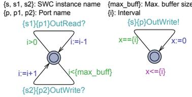
Figure 6: Schematic description realizing the communication between SWCs in form of a connector.
