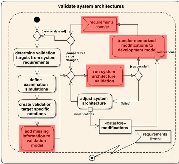
Figure 1: Process for system architecture validation
