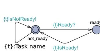
Figure 7: Schematic description of a UPPAAL TA representing the state of a task.
