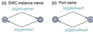
Figure 5: Schematic description of a UPPAAL TA realizing the behavior of the ports of a SWC.
