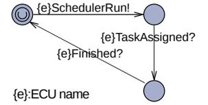
Figure 8: Schematic description of a UPPAAL TA realizing the behavior of the CPU.
