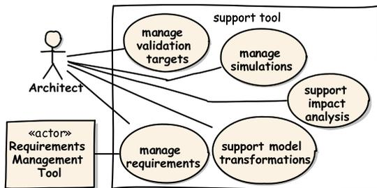
**Figure 5: Use case diagram of the support tool**
