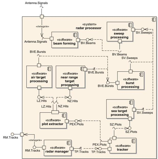
Figure 2: Software view of a simplified radar processor in development model
