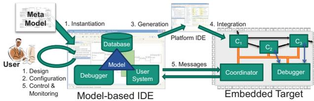
**Figure 3: Steps in the development using models for embedded platforms.**
