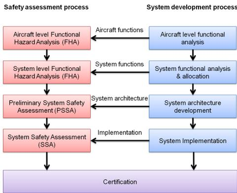
**Figure 1: Safety assessment process in relation to the systems development process**
