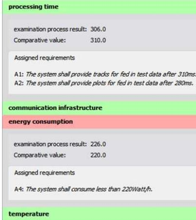
**Figure 6: Color-coded validation target overview according to validation status**
