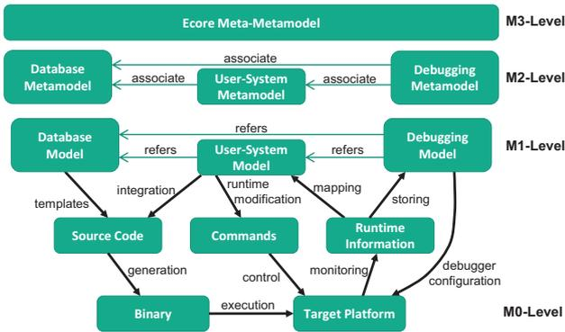
**Figure 1: Concept for model-based design, control and monitoring of embedded systems.**
