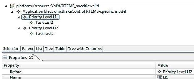
**Figure 10. RTEMS-specific model as an instance of the verification-oriented meta-model**
