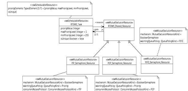
Figure 4. Excerpt of the RTEMS model
