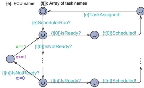
**Figure 9: Schematic description of a UPPAAL TA realizing the behavior of the scheduler.**
