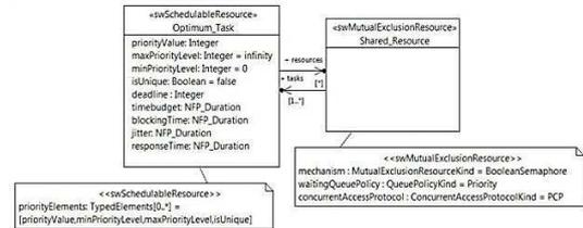
Figure 3. Excerpt of the Optimum platform model
