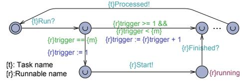
**Figure 4: Schematic description of a UPPAAL TA realizing the Task-Runnable mapping ④.**
