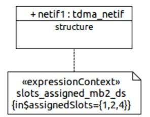
Through a constraint associated to a component instance
