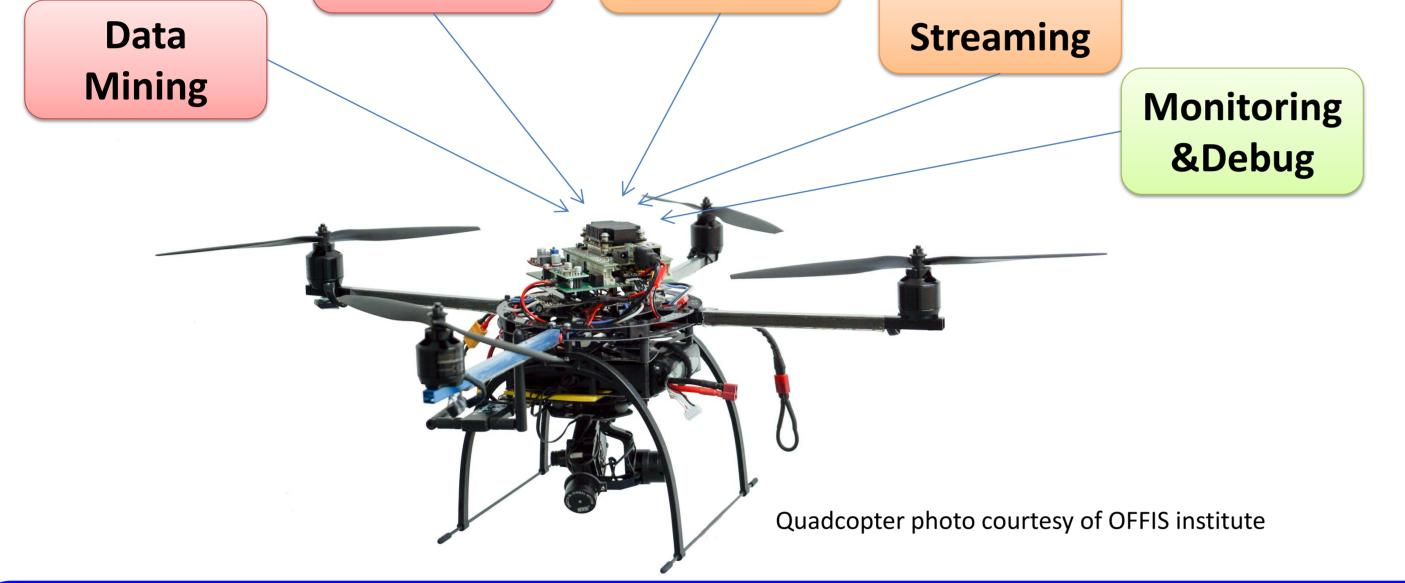
•Quadcopter system: safety-critical functionalities (flight algorithm, data mining, RC), mission critical functionalities (object tracking, video streaming) and non-critical functionalities (monitoring and debug)
