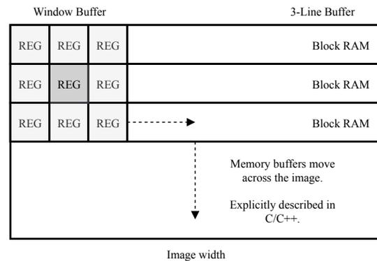
Fig. 5. Memory structures implemented to get efficient HLS implementations.
